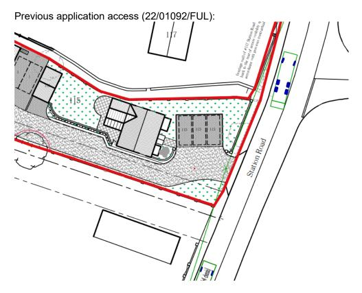
The LHA accepted the swept path analysis for refuse vehicles which are similar in scale to fire engines. The narrowest point on the access is 3.5m wide whereas a fire engine is typically 2.5m in width. Notwithstanding, it should be noted that building fire safety is covered by building regulations, and fire engines have hoses of up to 23m in length to reach into sites and this isn't a matter to consider as part of the planning application process.
